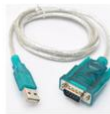
USB to RS-232 compatible serial port adapter
